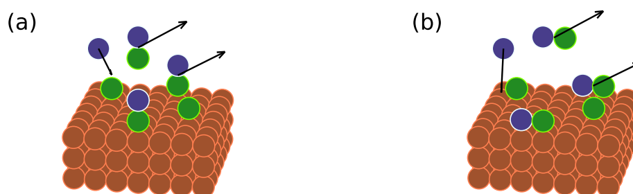
Figure 2.2: In the Eley-Rideal mechanism (a) one of the reactants interacts directly from the gas phase with an adsorbed molecule of the other reactant, whereas for the Langmuir-Hinshelwood mechanism (b) both of the reactants are adsorbed on nearby sites of the catalyst's surface.
