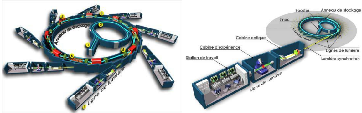
Figure 2.23: The storage ring of a synchrotron alternates between straight and curved sections (left). Insertion devices are situated along the straight sections, and deliver the synchrotron radiation to the beamline, separated in optical hutches, experimental end-stations and working stations (right).
